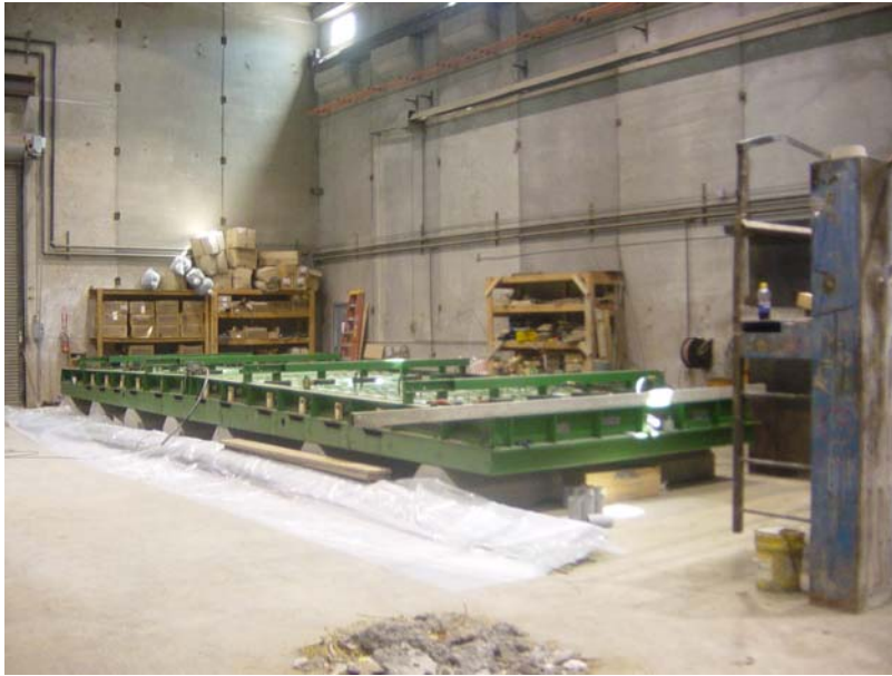
Figure 6: deck panel casting bed
